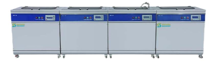
Loading → Ultrasonic Jet Cleaning (or Dynamic Shower Cleaning) → Dynamic Shower Rinsing (or Jet Bubble Rinsing) → Jet Bubble Rinsing (or Dynamic Shower Rinsing) → Recirculation Hot Air Drying → Unloading
